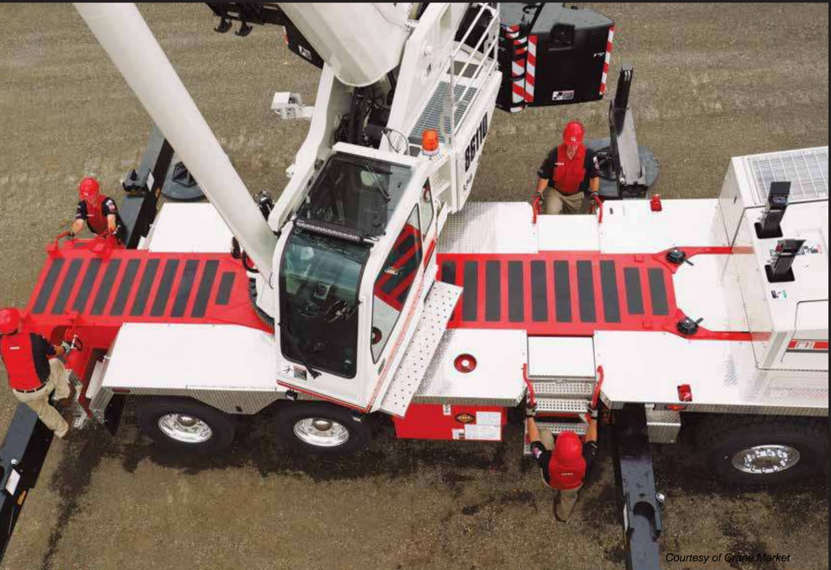
Access to the operator's cab and engine compartment is superb with strategically located ladders and steps .
