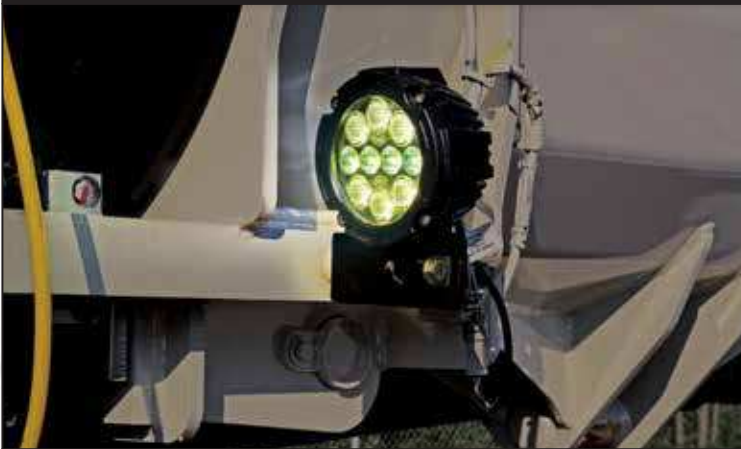
Single boom flood light (detail)
