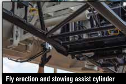
New efficient fly pinning design focuses on ease of assembly/disassembly
