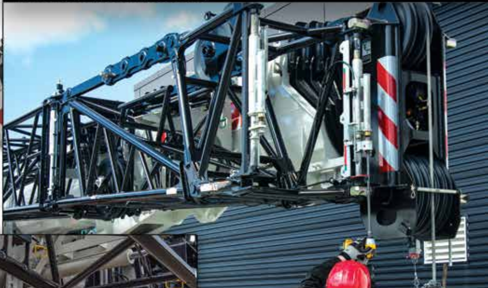
New efficient fly pinning design focuses on ease of assembly/disassembly
