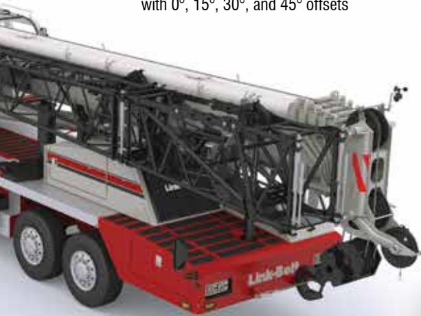
Quick reeve boom head eliminates the need to remove the becket when it becomes necessary to change the reeving
