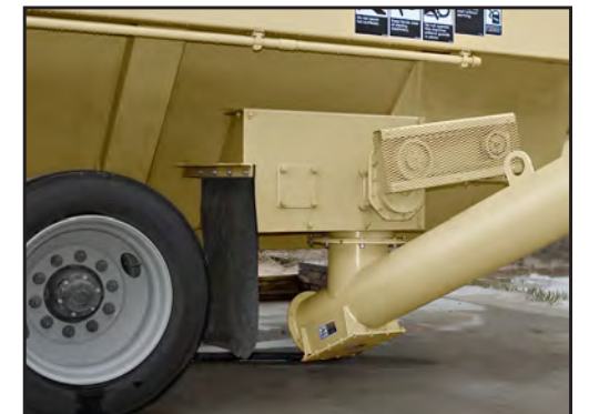
Captured baghouse fines are returned to the mix by a dedicated auger.
