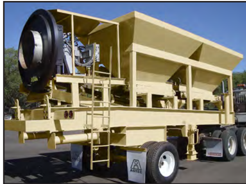
Optionally, the aggregate system can be made as a detachable unit for maximum portability.
