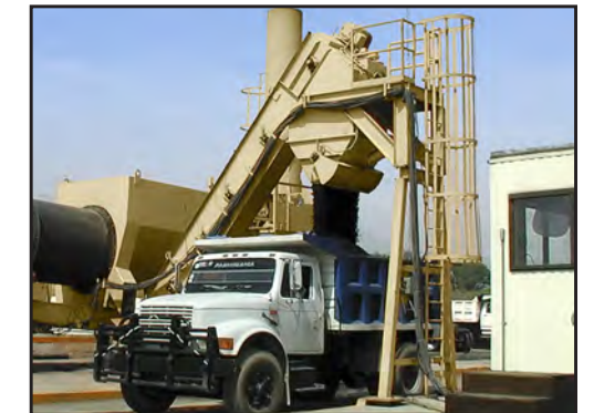
The drag conveyor features an integral hopper that serves as a surge bin for loadout.
