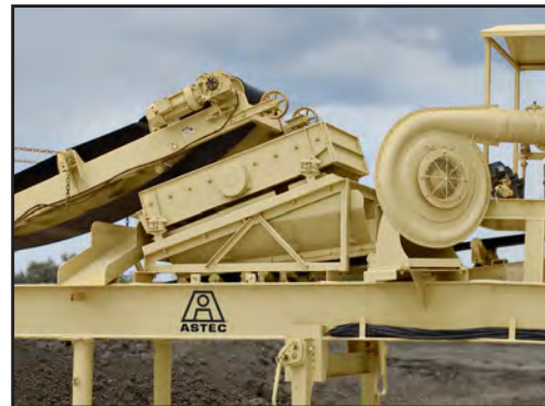
The scalping screen removes and discharges any oversized material from the aggregate.
