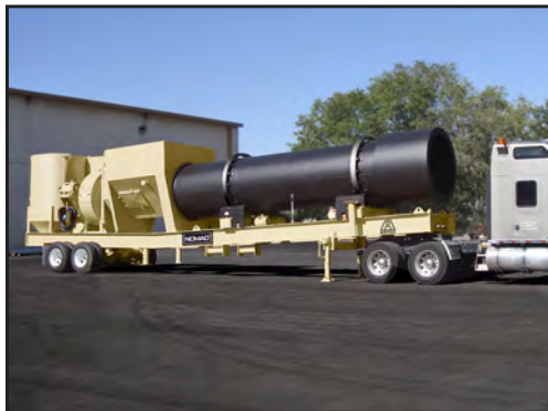
Drum mix unit shown with optional detachable aggregate system removed.
