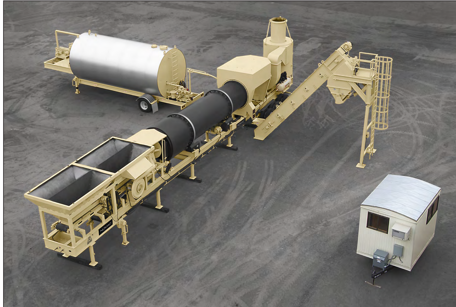
Optionally, the aggregate system can be made as a detachable unit for maximum portability.
