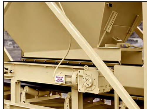
Adjustable discharge gates and feed belts with variable-frequency drives (VFDs) allow precise control of aggregate size & feed rates.
