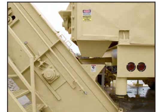
Finished mix is discharged into the base of the plant's drag conveyor.
