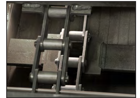
Drag conveyor features a chrome-carbide steel liner for superior durability.
