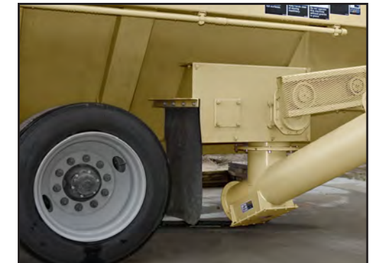
An auger returns captured baghouse fines to the twin-shaft coater for mixing.
