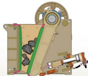
Clearing is achieved using push button controls. Cylinders retract the toggle beam and pitman, allowing the stone to fall.
