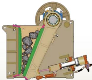
During normal crushing, hydraulic cylinders hold the toggle beam forward.
