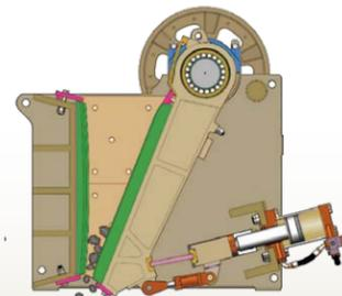
Cylinders push the toggle beam and pitman forward, crushing the remaining stone. Cycling through this process a few times clears the chamber.
